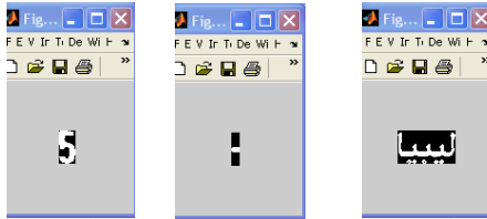
Figure 5: Sub-images of letter, number, and word separated from plate
