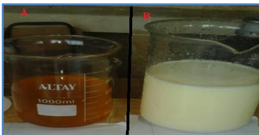
Fig. 5 Biodiesel product (A) before washing and (B) after washing with distilled water.
