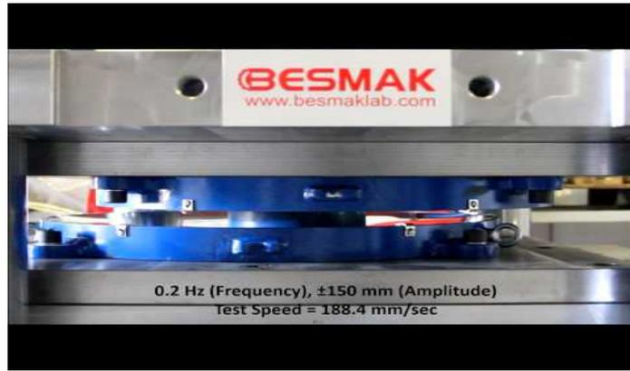
**Figure 5: Sliding Base Damping System**
