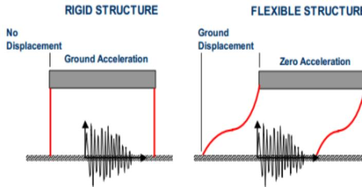
**Figure 8: Transmission of ground movement**
