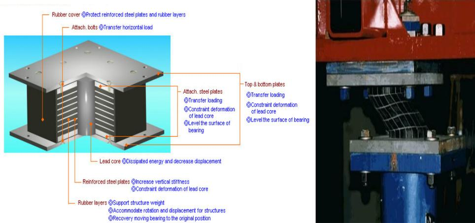
**Figure 3: Elastic bearing and its shear twisting**
