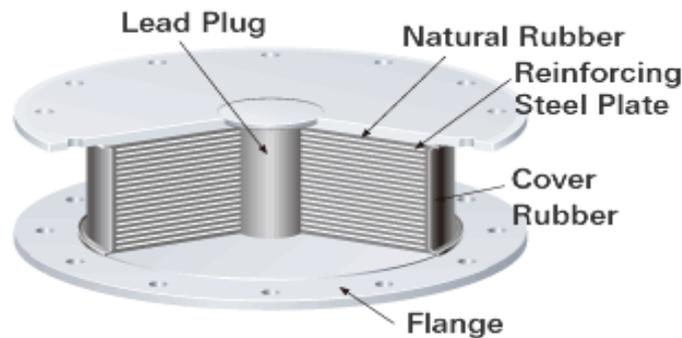
Figure 4: Components of Lead-plug elastic bearing
