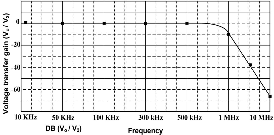
Fig. 6: Low - pass frequency response of the filter
