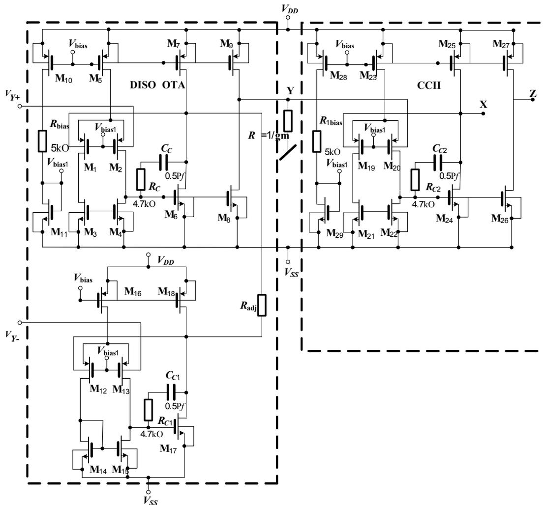
Fig. 3: CMOS Implementation of DVCCII+ by Bulk-driven current conveyor and by OTA.
