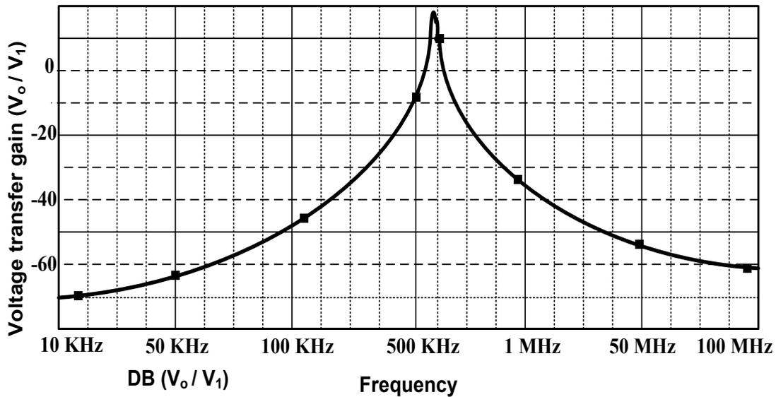
Fig. 7: Band - pass frequency response of the filter
