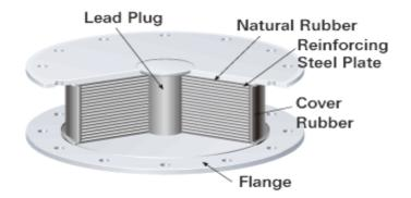
Figure 4: Components of Lead-plug elastic bearing
