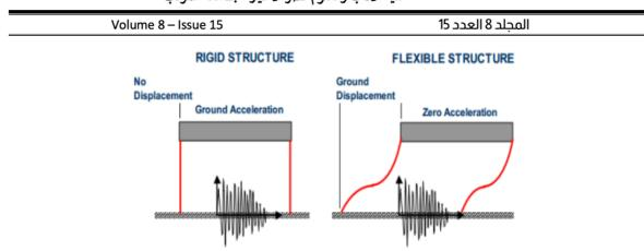
Figure 8: Transmission of ground movement
