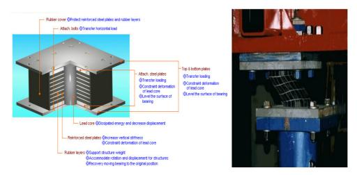
Figure 3: Elastic bearing and its shear twisting
